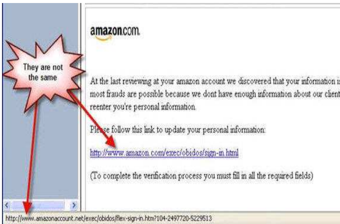
Figure 1: Early iteration of an intervention. When people clicked on a link in one of our training emails, it would bring up a screenshot (above) of the web browser showing that the URL they thought they clicked on was not the same as the URL that the web browser would go to (web browser status bar).
