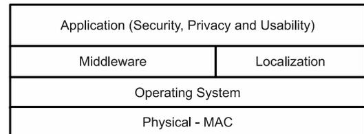
Figure 1: Simplified modular architecture of a programmable phone
